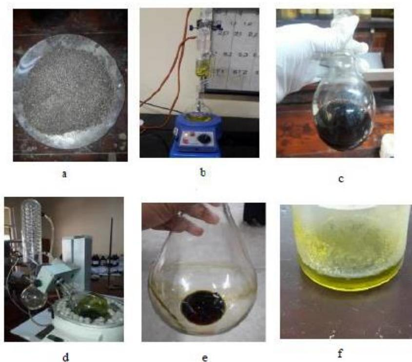
**Figure 1:** Stepwise process of extraction (a) Ground algal biomass, (b) Oil extraction by soxhlet apparatus, (c) Oil and solvent mixture, (d) Solvent evaporation by rotary evaporator, (e) Extracted oil, methanol and NaOH, (f) Unpurified biodiesel.
